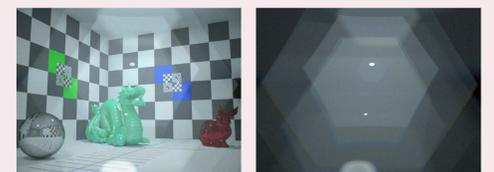
By saving the result in the forward light tracing pass, the lens flare can be examined separately from other effects.
