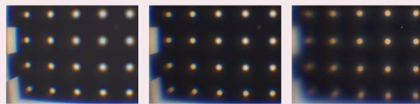
Unequal focus near the border is caused by spherical aberration and field curvature. The color shift of the marginal circles in the defocused left version is called lateral color originating from varying magnification over all wavelengths.
