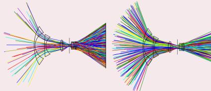
Path plot for a Muller [Smi05] fish-eye at f/8. The aperture has only 1.8mm diameter. Ray passage rate is 10% without (left) and 82% with pixel pupil sampling (right).
