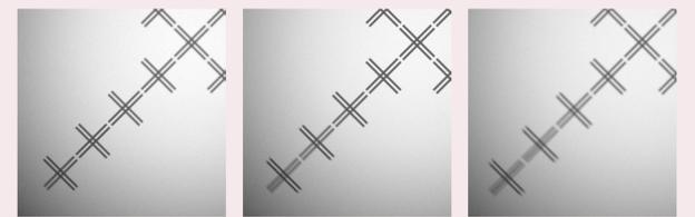
Astigmatism and field curvature observed for a Petzval[Smi05] design lens at different image distances. The shown pictures are lower left corner crops of an astigmatism cross test pattern, in front of, in, and behind the plane of focus. Tangential structures in the marginal regions stay rather focused, the sagittal lines towards the center become blurred.
