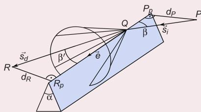
Aveneau and Mériaux proposed using Keller's Geometrical Theory of Diffraction in an image rendering setting. Contrary to their approach, we are explicitly sampling the diffracted path directions inside the Keller Cone, the space of all valid diffraction directions. An appropriate diffraction coefficient for unpolarised light can be found in [AM99].
