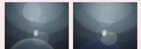
Examples clearly showing how a single lens coating suppresses specific lens flare parts.
