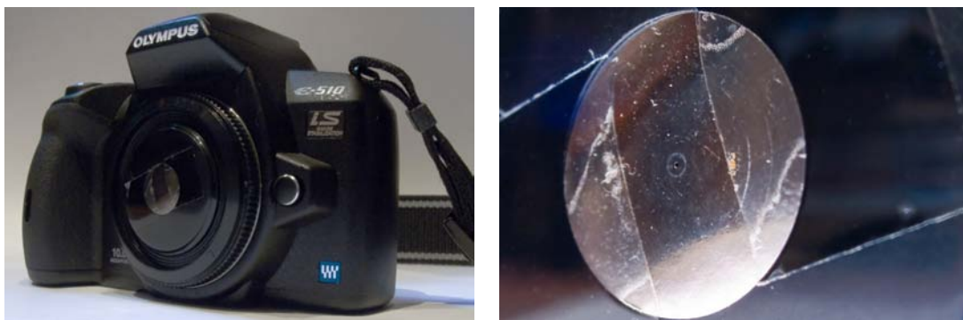
(a) Modern version with 0.22mm diameter hole in 0.02mm thick plate mounted on DSLR back
