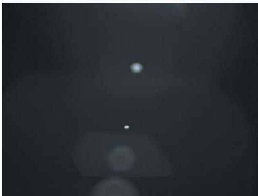
(c) The flare produced by the lens appears as considerable veiling glare, which destroys the scene contrast. The aperture ghosts are faint.
