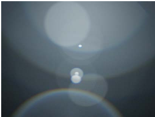
(b) As the lens has no aperture, all flares are round shaped. The high variance region in the lower middle should result in a similar circle like the large rainbow around, but this one seems to have horrible paths.
