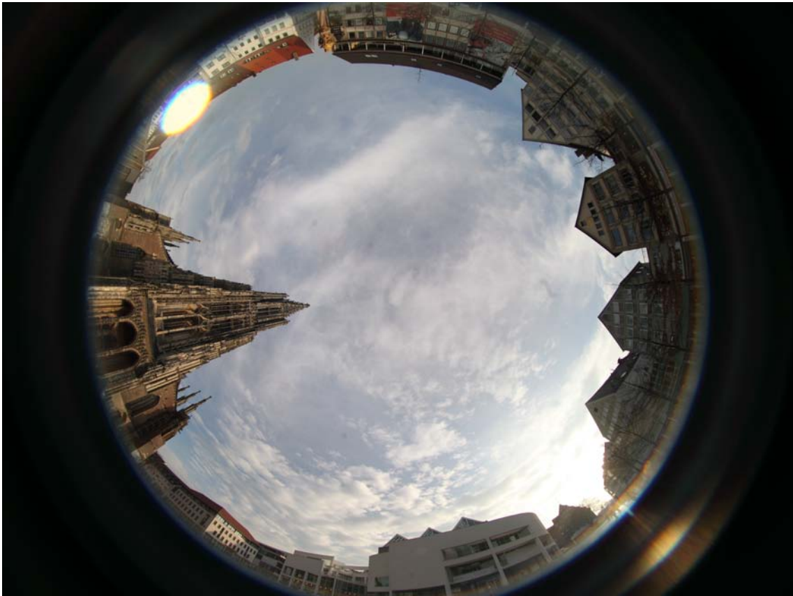
Figure 3.18: This panoramic fisheye picture of the Ulmer Muensterplatz , taken with a Peleng 8mm circular fisheye lens on a Canon 5D MKII at f/16 shows various imaging defects, mentioned in this chapter. What first catches the eye is the deliberate distortion which is needed to reach the 180^\circ field of view. In the upper left corner there is a bright ghost of the sun, formed behind the aperture stop, thus it has the angled diaphragm shape. Explicit chromatic aberration on the edge of the ghost is visible, also along the whole image border. In the lower right corner we see glaring stray light which emerges from reflection of the sunlight inside the body.
