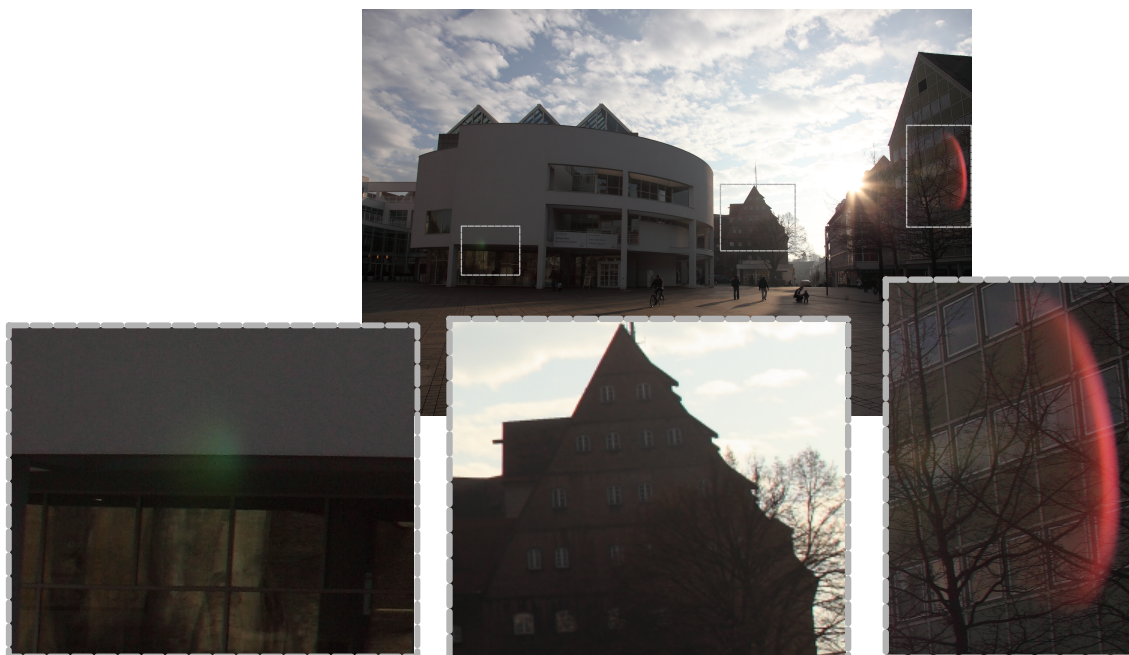
Figure 3.17: Picture taken with a Canon 5D MKII and Canon L Series lens. The two different colors of the lens flares reveal a bit about the different used coatings. The mid enlargement of the house wall shows another alerting effect. The contrast of the wall looks considerably reduced, which can happen due to stray light in the lens barrel or veiling glare. The latter mentioned is a lens flare that spread over the whole image area.
