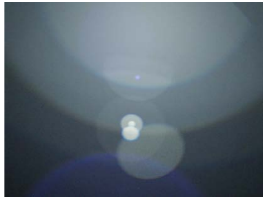
(c) The second element in the lens was coated from both sides and gives this result. Although not visible here, the RGB average image brightness increased by (+8.8%, +10.0%, +3.8%).
