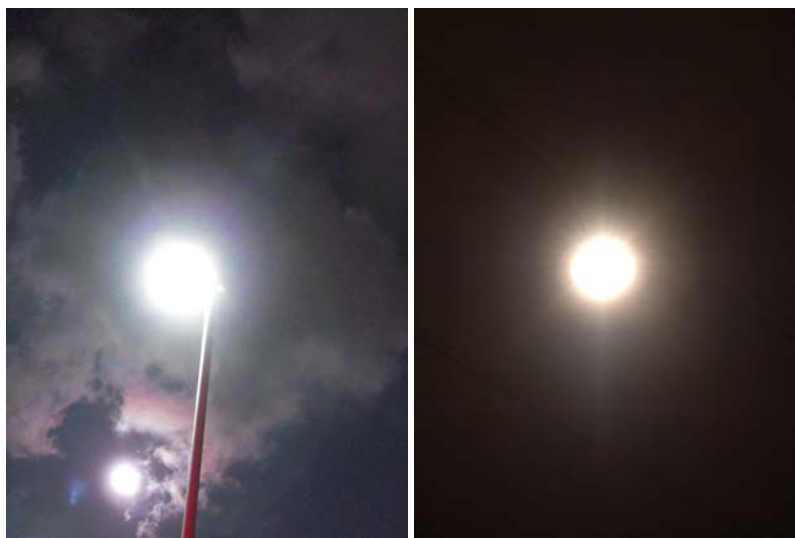
Figure 5.10: Real glare streaks formed by aperture edges. On the left side, above the lantern, two main streaks can be identified. On the right side, there are many short streaks, arising from the border ring of the spot light. But also main streaks in all directions are recognizable. Also compare the given examples with Figure 3.17, where the shot towards the sun produces large streak bands. Left photo by courtesy of Katharina Schwarz.
