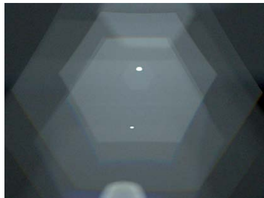
(d) In the stopped up version, the veiling glare begins to form aperture ghosts in the image center. Both spots concentrated to visible ghosts of the light source.
